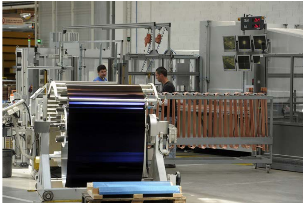
The joining partners: on the left, the coil with the coated sheet; on the right, the trolley with the meander pipes
