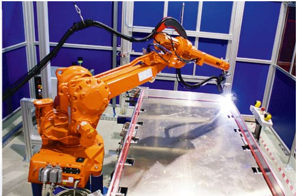
A system from DTEC in action: laser welding of a collector frame
